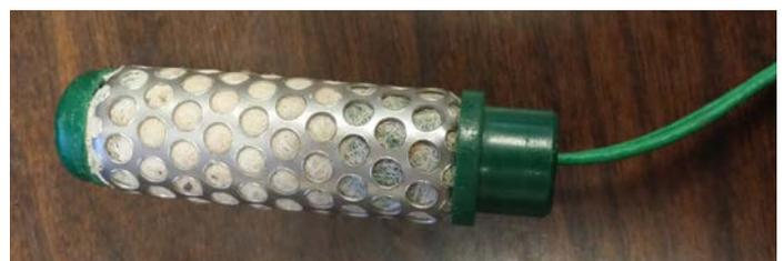
Figure 2: The Irrometer Watermark is an example of an electrical resistance block.
