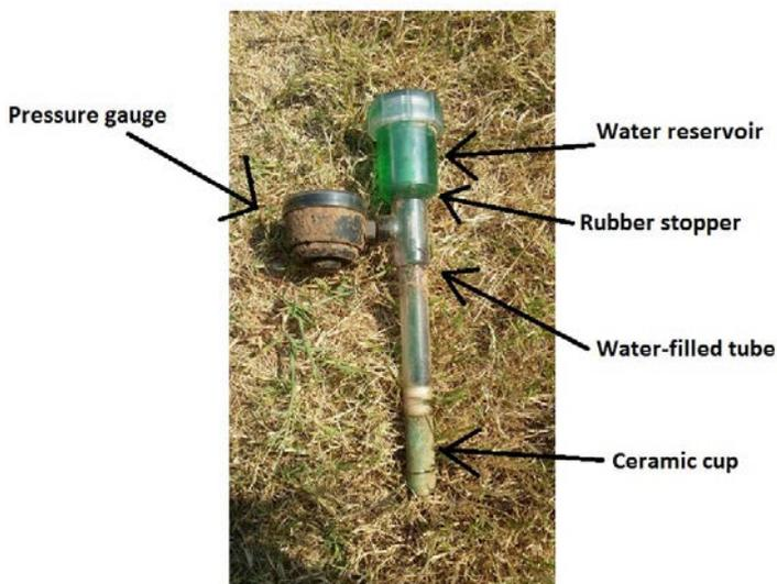
Figure 1: Diagram of a tensiometer.
