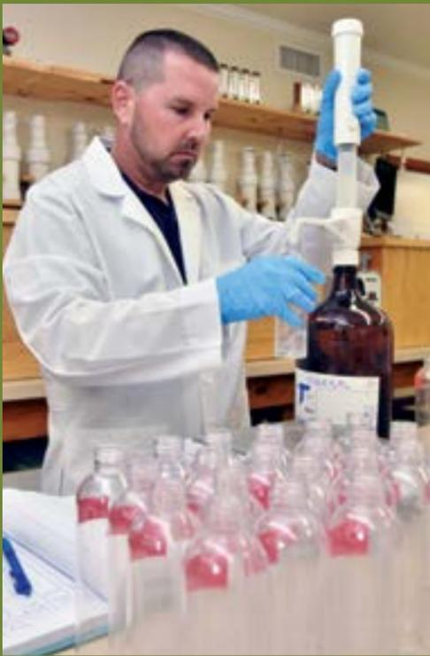
Dustin Harrell prepares a sample to be tested in a laboratory with an experimental urease inhibitor to reduce ammonia volatilization. The research uses different soils from across the state, with different temperatures and varying durations. The work is aimed at showing growers potential benefits of a urease inhibitor before flooding.
