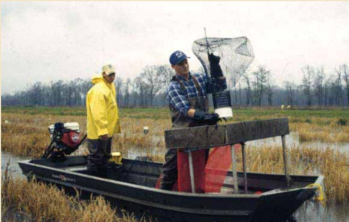
Figure 8.6. Crawfish harvesting boat powered by Go-Devil® propulsion unit.
