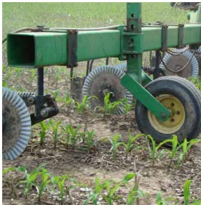
*Figure 4-3. Side view of liquid fertilizer applicator in a conservation tillage system. The fluted coupler opens a narrow furrow in which liquid fertilizer is dropped behind the knife that follows the couler.*
