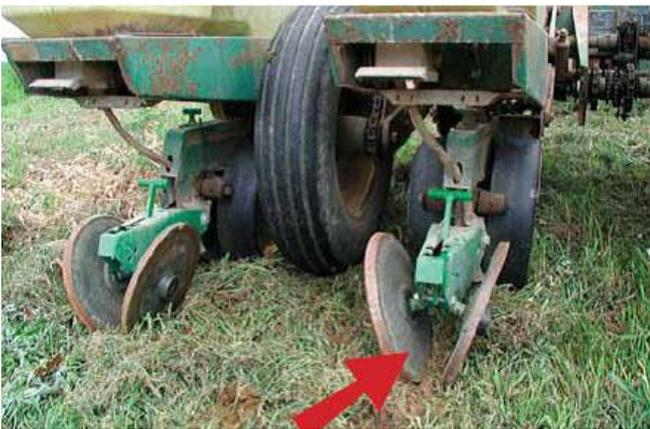
Figure 8-10. Cast-iron closing wheels.
