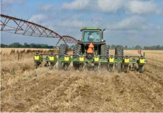
*Figure 1-6. Special row cleaning tools are usually not needed for planting into crop residue but, when biomass production is very high, such devices may improve seed placement and stand establishment.*
