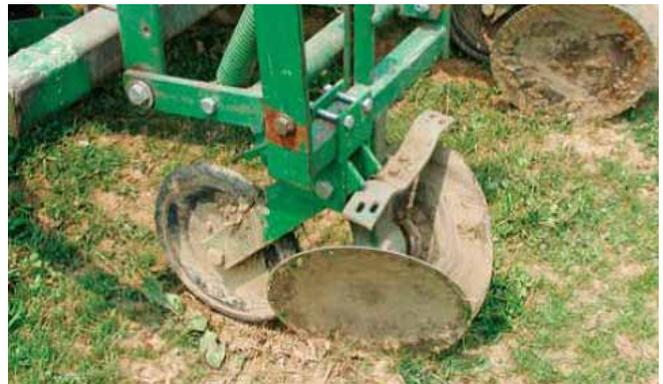
Figure 8-5. Residue cleaners with concave disks.
