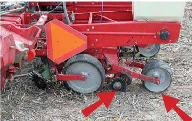
Figure 8-11. Case-IH rubber closing wheel.
