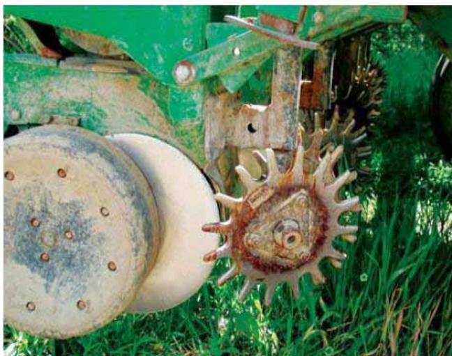
Figure 8-3. Residue cleaners with straight fingers.
