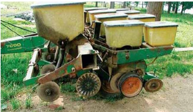
Figure 8-8. A planter mounted with a bubble couler.
