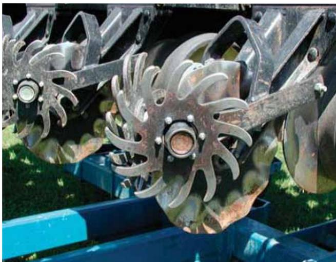
Figure 8-2. Residue cleaners with curved fingers
