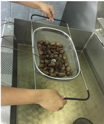
*In-shell pecans being treated with hot water during the study at LSU AgCenter.*
