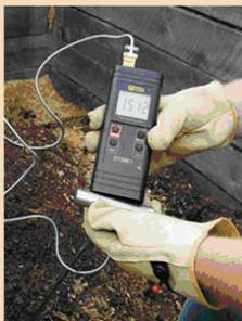
One example of a temperature probe. (Notice the temperature of 151°F.)
