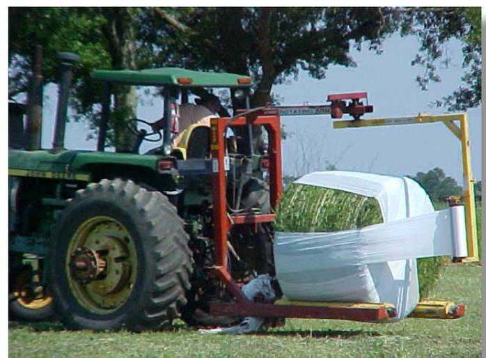
**Figure 2. Picture of in-line baleage wrapper. Photo credit: Dr. Dennis Hancock, University of Georgia.**
